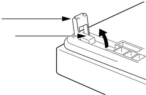
Two larger, detached riser brackets elevate and angle the unit more than the foldout legs. Use moderate force to snap them into the bottom panel as shown.
