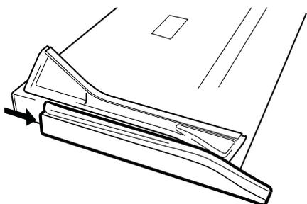
2 Press the tabs to release the riser brackets.
